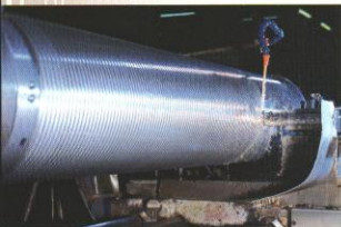
The drum is being machined. The drum represents a major component of the hoist.
