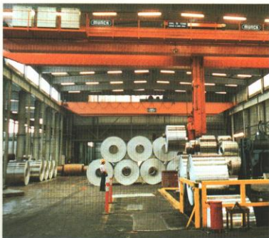
Munck -Mobilstak- is a speciality by Munck. The Mobilstak can be equipped with special lifting attachments to suit different products which are to be handled. Photo shows -MOBILSTAK- at one of the Norsk Hydro plants in Norway.
